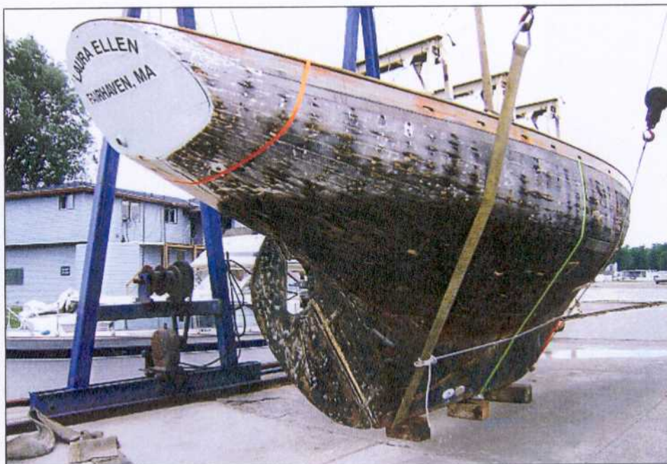
Laura Ellen, a junior Bluenose, in the slings at Ecarte Marina. The keel was submerged to swell up the timbers in the keel's deadwood.
